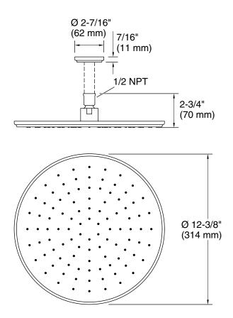
Technical InformationAll product dimensions are nominal.Drain included:NoShowerhead/Body Spray:Rated maximum2.5 gal/min (9.5 l/min)flow:Pressure:80 psi (5.5 bar)
